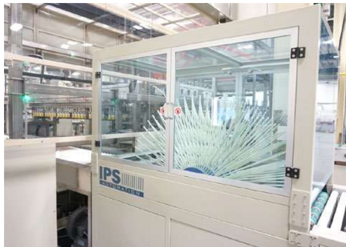
IPS panel accumulator.
