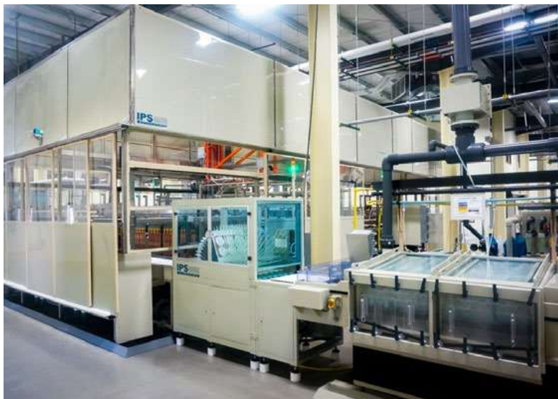
IPS fully automated plating line.
